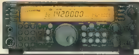
TS-570D HF base station
